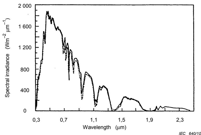
NOTE Optical depth of aerosol extinction 0,1 (solid line) and 0,27 (dashes), respectively.
